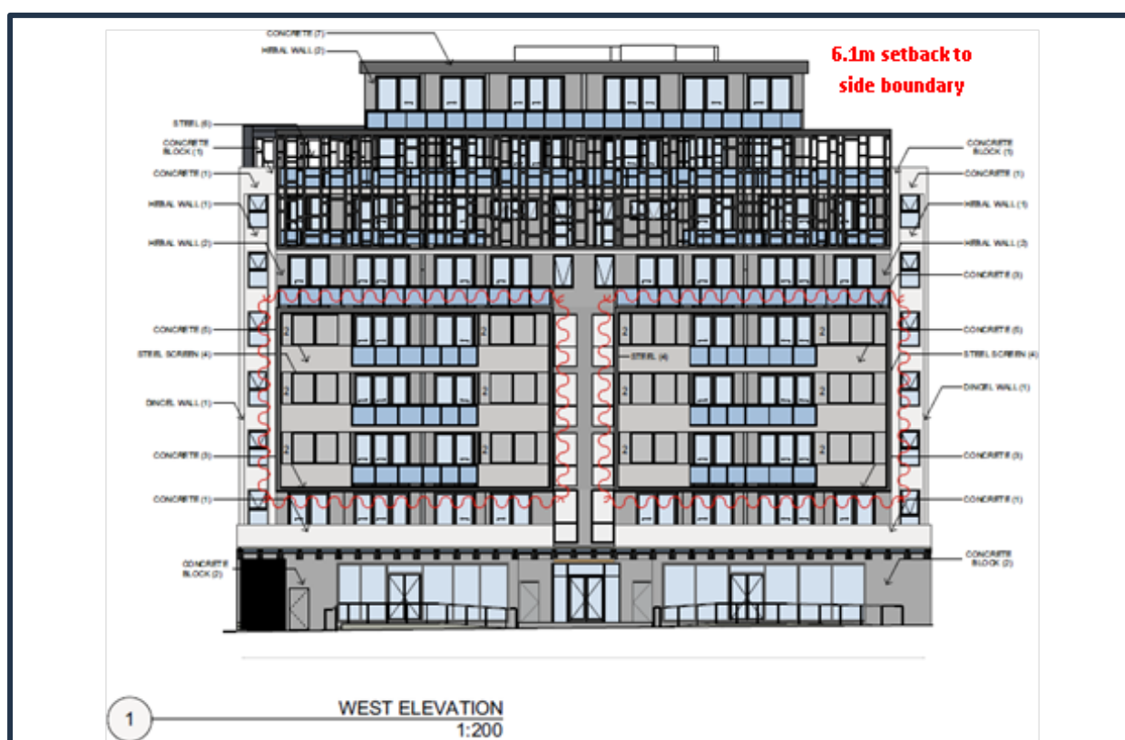
Figure 1: Western elevation of adjoining mixed-use building at 166-176 Terminus Street, Liverpool approved under DA48/2015. Level 7 & 8 achieve a 6.1m setback to sites south-western boundary.
